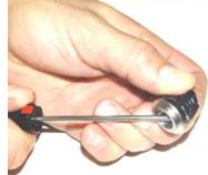
INSERT A SMALL SCREWDRIVER BETWEEN THE CHECK VALVE POPPET AND VALVE CAGE. CAREFULLY TWIST THE SCREWDRIVER UNTIL POPPET COMES APART.
