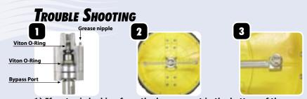
1) If water is leaking from the bypass port in the bottom of the rotary head: Inspect the viton O-Ring in the rotary head. 2)Rotary Arm doesn't spin:
