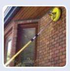
Attach to a longwand for cleaning hard to reach surfaces. Connect to longwand using the QC fittings on the longwand and Whirl-A-Way. Ensure the M22 hose is connected properly before use.
