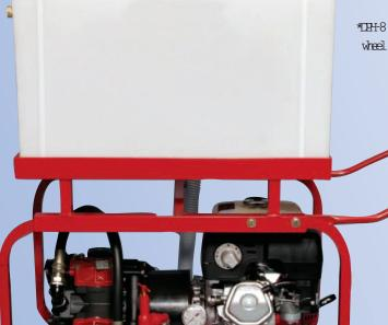
\*DH-8 Shown with optional wheel and handle kit. he **DP Series** hydrostatic test pumps are large volume, medium pressure units, with flow rates up to 56 GPM and pressures up to 600 PSI. Designed to quickly fill and test lines up to 96" in diameter. Unique to the diaphragm pumps are their ability to handle up to a 10% chlorine solution, and can be run dry without damage to the pump.
